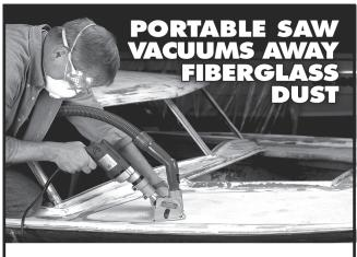
Kett's KSV-432 Vacuum Saw has a 2 1/2" carbide blade for fast cutting of fiberglass with
